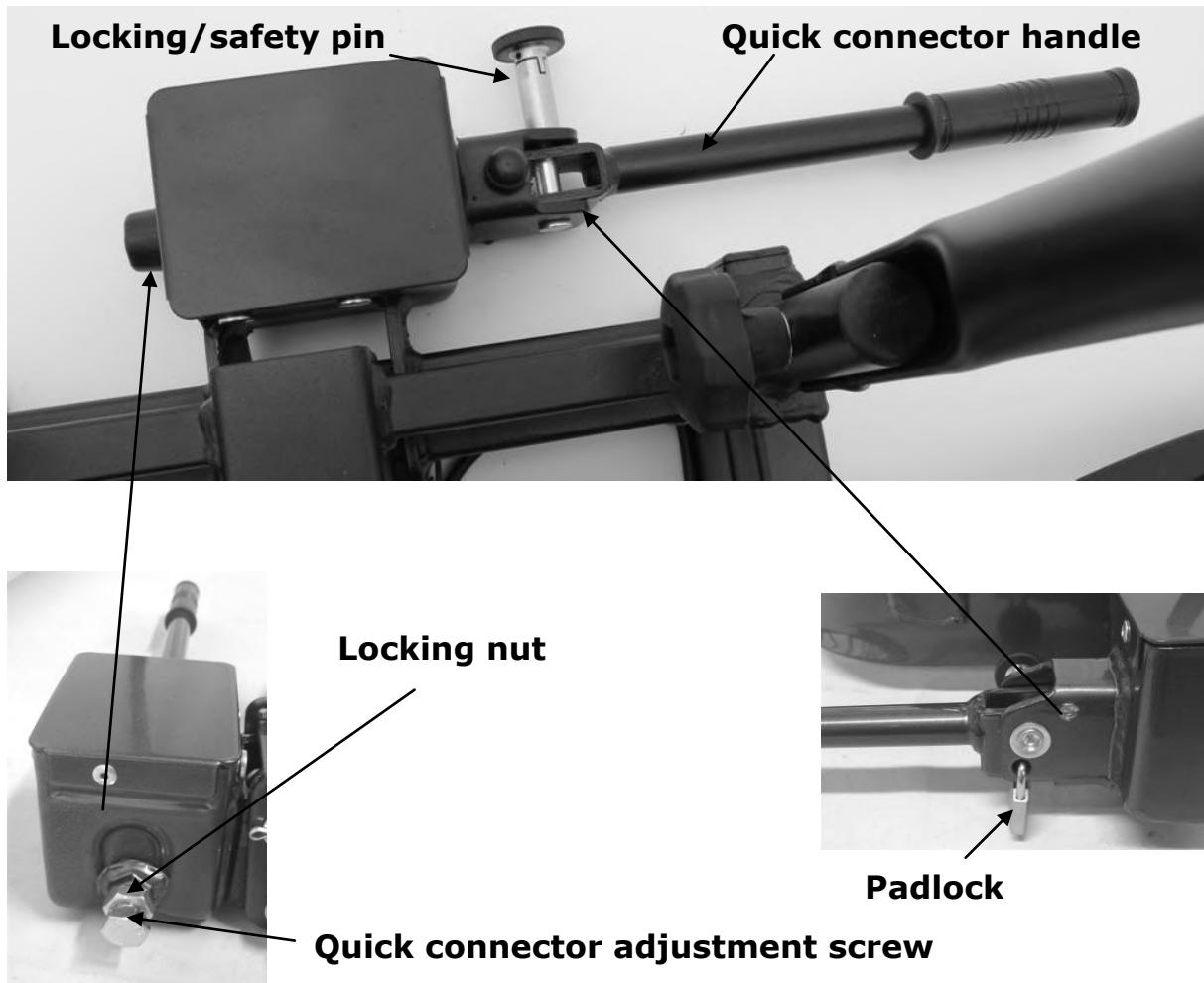
The quick connector consists of a case mounted to the bike carrier and a lever. Using the lever, you can close and open the quick connector.
