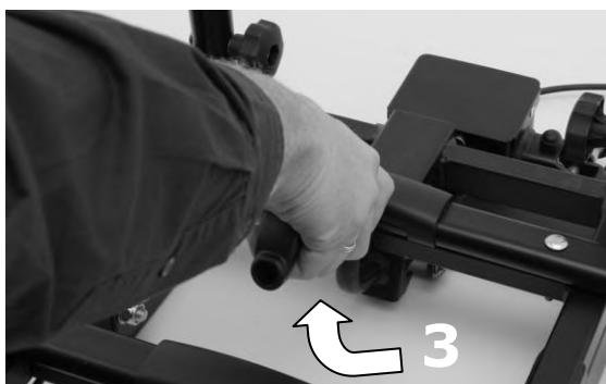
With one hand, keep a firm grip on the U-frame so that the carrier cannot fall down in an uncontrolled movement. With the other hand, pull the handle of the tilting mechanism up to unlock it (3). It is now possible to tilt the carrier.
