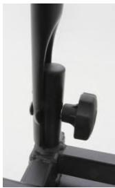
Slide the U-frame against the outside of the U-frame holders of the base frame. Secure this U-frame with the supplied carriage bolts (M8x60), washers and plastic rotary knobs.
