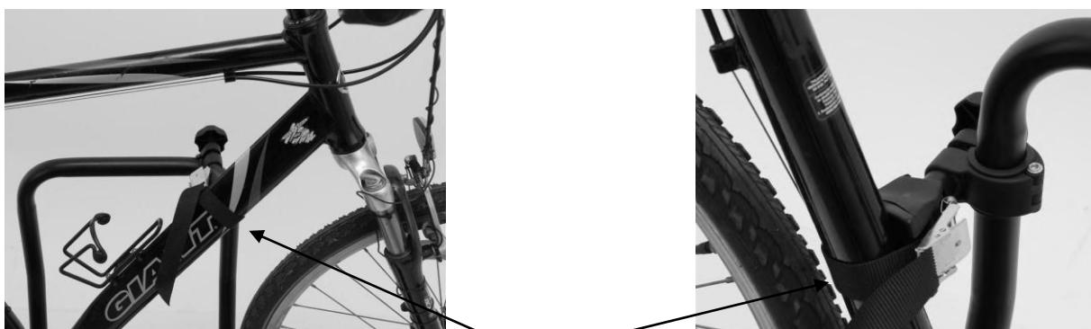
Use the straps to secure the bikes. With these straps, any bike can be secured easily without placing a load on the bike crank.
