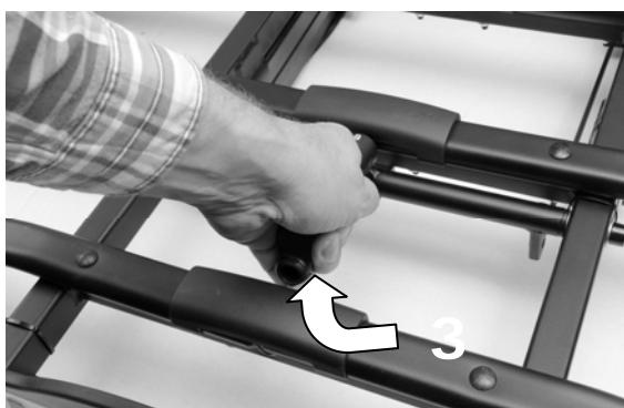
With one hand, keep a firm grip on the U-frame or bikes so that the carrier cannot fall down in an uncontrolled movement. With the other hand, pull the handle of the tilting mechanism up to unlock it (3). It is now possible to tilt the carrier.
