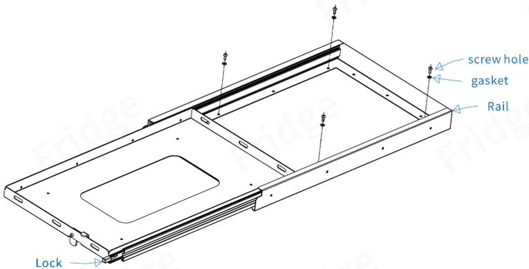
3. Fix the refrigerator on the slide with tightening belts.
